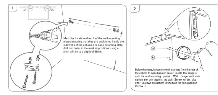
Note: - There are two sets of hangers on the back of the column. This allows the column to be hung so that the door opens in the desired direction.
