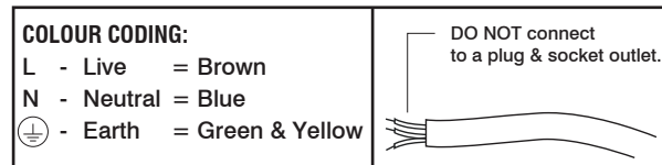
WIRING DIAGRAM - MAINS SUPPLY
