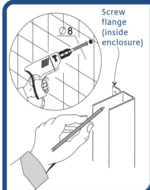
Measure & mark wall rail Positions. Mark fixing hole positions, drill & plug walls. Having decided required handing, **AFFIX DOOR SIDE WALL RAIL ONLY AT THIS STAGE.**
