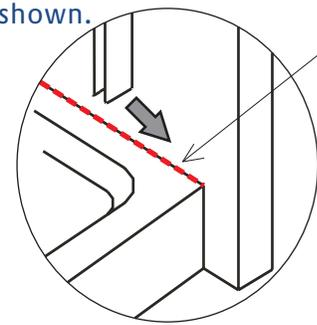
Ensure continuous silicone sealant bead before fitting wall rails
