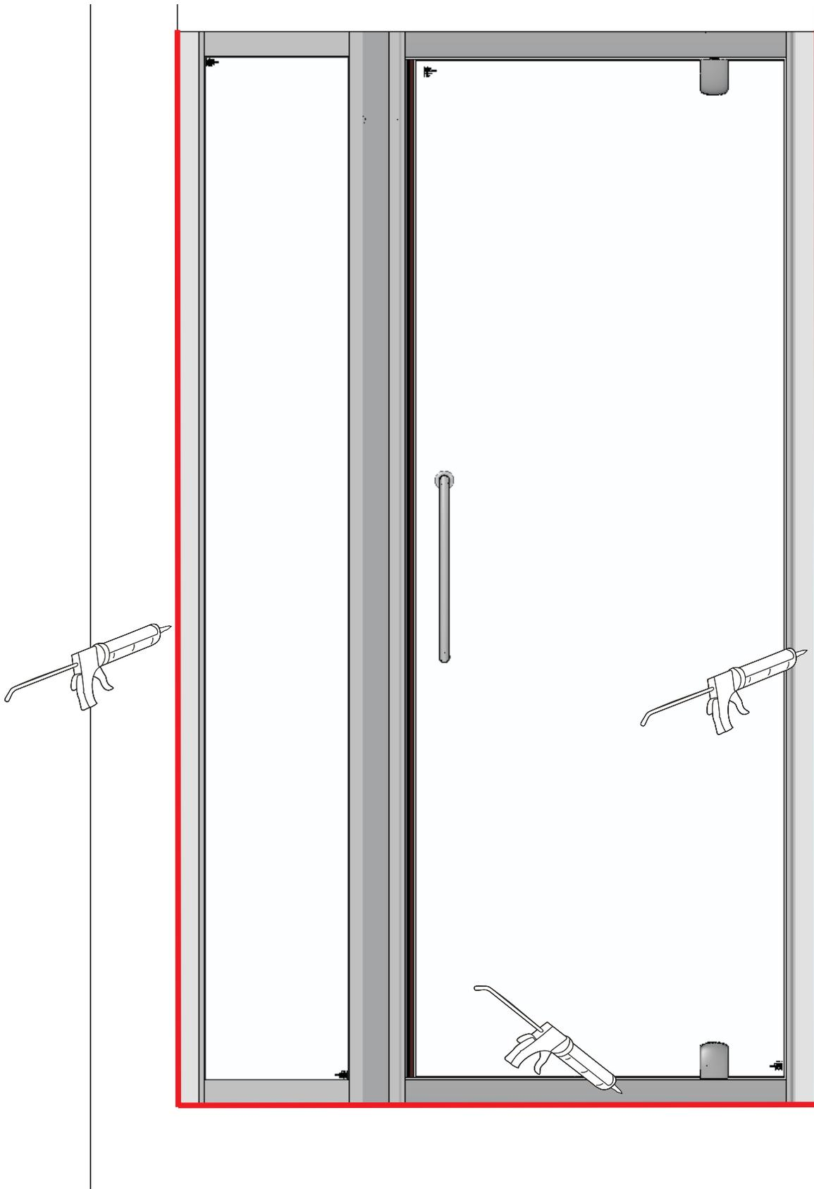
Use of good quality silicone sealant & cleaning / degreasing of all joint areas is recommended.
