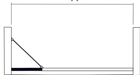
Lakes Inline panel 'pack' for use in line with standard shower doors. Ensure tray is correctly levelled & that tray / wall (tile) joints are sealed & cured over entire length of tray sides (See Fig A) prior to fitting enclosure. **DO NOT SEAL TRAY EDGES UPTO A FITTED ENCLOSURE !**
