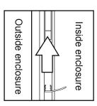
8- Push seal No.8 the samaller fixed panel seal onto the large fixed panel and seal No.9 the larger of the fixed panel seal onto the small fixed panel where the door closes onto
