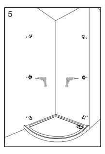
5 - Remove the assembly and drill the marked points using an 6 mm masonry drill bit, once this is done insert 6 x wall plugs into the holes.
