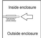
9-Attach the handle making sure that the rubber washers that come with the handle are placed between the handles and the galss.
