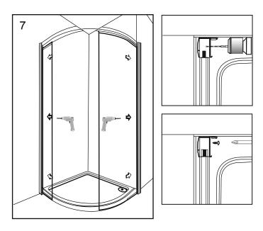
7 - Whilst ensuring that the bottom of the assembly is held snug to the shower tray and that all parts are level and upright, fix the assembly to the wall channels by drilling through the pre drilled holes in the wall channels into the profiles of the fixed panels using a 2.75 mm metal drill bit. Then secure using 8 x ST3.5x10 short screws (4 per wall channel).
