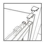
11 - Once you are happy that the installation is correct and that the doors are running smoothly, push the cover caps onto the top of the wall channels as shown, (smaller top cap first followed by the larger wall channel top cap).
