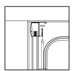
6 - Reposition the assembly and fix the wall channels to the wall using 8x ST4x30 long screws (4 per channel)
