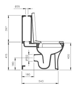
DIAGRAMS NOT TO SCALE  $\mid$  ALL DIMENSIONS IN MM TOLERANCE OF  $\pm$  5MM  $\,$  ALL PRODUCTS CONFORM TO BRITISH STANDARDS
