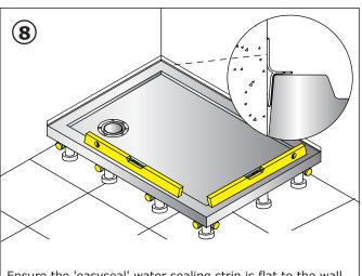
Ensure the 'easyseal' water sealing strip is flat to the wall. Place the tray into position and level both ways using the legs. After the tray has been levelled adjust all the inner feet to stabilise the tray. When level fix these legs to the floor with silicon sealant or 'no more nails' type adhesive.
