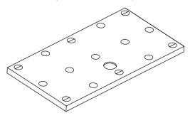
Turn the tray over and use the cardboard packaging as a protective mat. Note the circles that have been marked to indicate feet position. The symbol  $\ominus$  indicates where you should fix the feet with the panel fixing rod, but for the symbol  $\bigcirc$  you will only use four of these positions and the other two would be supplemented with the feet without the panel fixing rod.
