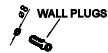
Step 5: Drill two holes of \varnothing 8\text{mm} with depth of 40mm, tap in wall plugs.
