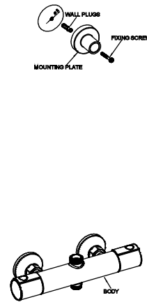
Step 5: Place mounting plate against wall and make markings for a hole. Drill a hole of 25mm with depth of 45mm. Tap in wall plugs, then fix the mounting plate against wall with screws.
