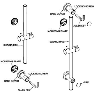
Step7: Fix bottom base cover onto the mounting plate, place sliding rail into base cover in a proper position, then turn the locking screw with allen key to tighten.
