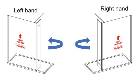
Step 1 – Remove swivel panel from packaging. Install the swivel panel in required orientation. Product is reversible and no brackets need to be removed to change handing.
