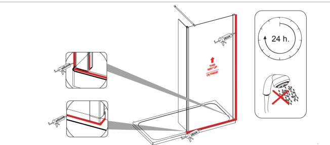
Before sealing make sure all surfaces are clean, dry and free from any residue such as grout. Use quality silicone sealant and applicator gun to fnish the wetroom panels.
